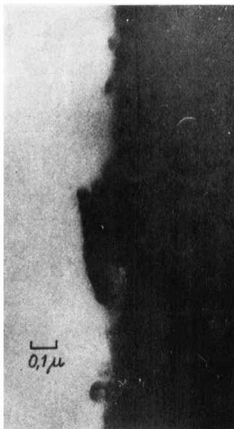
FIGURE 3 Electron photomicrograph of transverse section of film of poly(butyl methacrylate) and poly(vinyl chloride), doubled at 210–220°.
